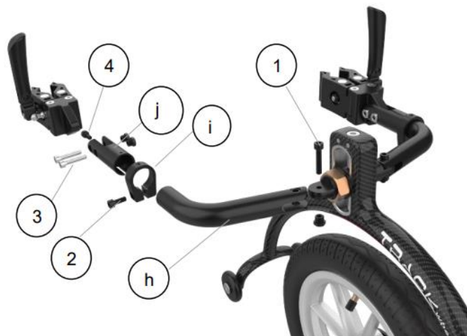
Figure 22. Exploded Picture of Adjustment Arm Mechanisms
